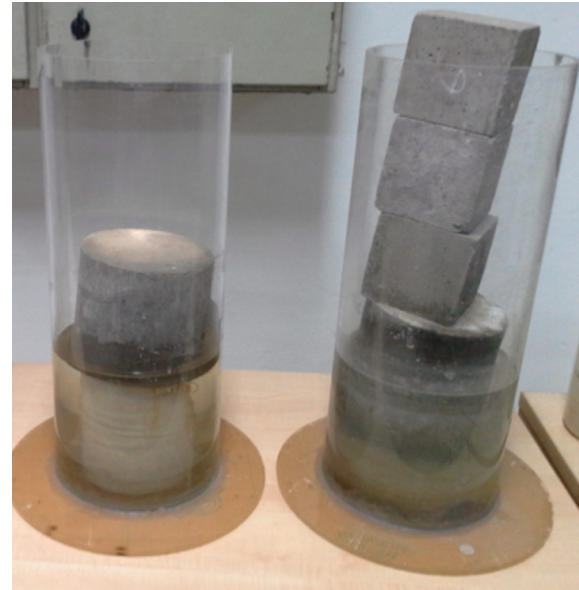
Fig. 3. Surcharge loading application on top of column-shape geo-bag filled with chemically treated MC.
