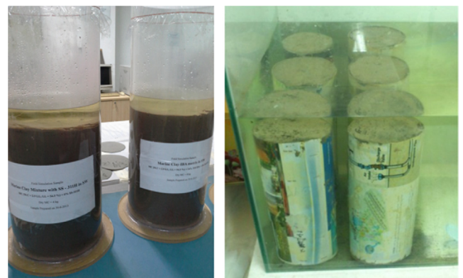
Fig. 8. Pure chemically stabilized MC samples under sea water.
