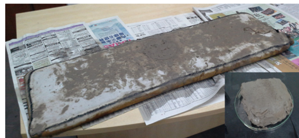
Fig. 4. Beam-shape sample after 1-m CPCM2 process.
