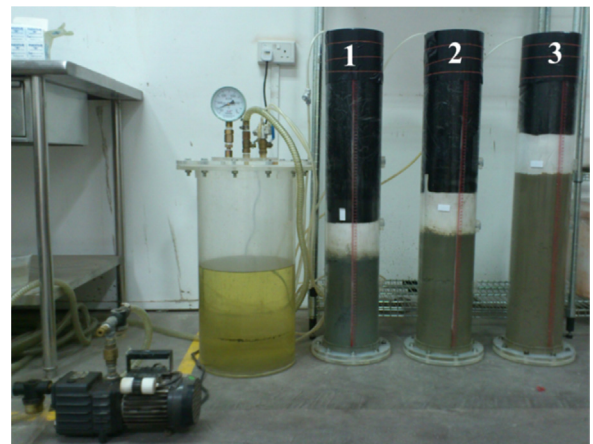
Fig. 1. Experimental setup of vacuum preloading application. (a) Sketch illustration of vacuum preloading experiment, (b) Vacuum preloading experiments using large 3D consolidation cell.
